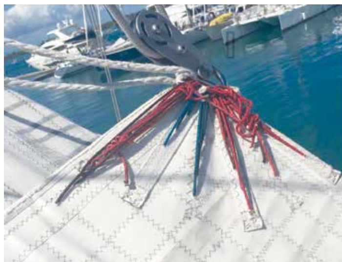
The repair to the head car of the mainsail. This small failure in the worst place, caused us to go east about instead of west about. I think we are one of the few yachts to have sailed circumnavigated Australia via Hong Kong. This repair lasted 2,000 nautical miles. Dyneema cordage is a yachtsman's fencing wire
