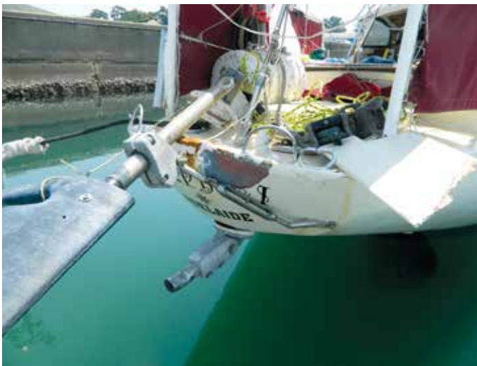
The damaged transom
