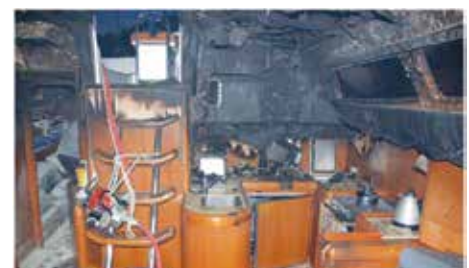
A faulty dehumidifier wrote off this boat. Photo: Yachting Monthly
