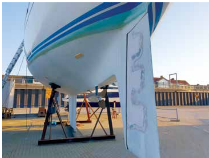
Repaired rudder and dyna plate for HF
