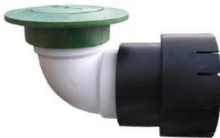
The NDS drainage emitters act as the discharge point for a drainage system. The patented spring-loaded cap pops open with the pressure of water flowing through the drainage pipe then closes as flow diminishes.
