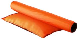
This porous cylindrical tube is placed in front of curb inlets and median inlets and extends beyond the inlet opening for full gutter protection. The Dandy Curb is made from orange high visibility monofilament fabric and has an attached aggregate pouch to weight it in place.
