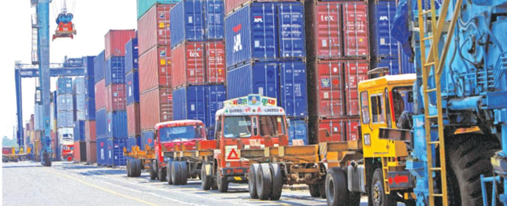
TRACTOR-TRAILERS WAIT IN LINE TO LOAD CONTAINERS AT THE CONTAINER YARD. RAIL-MOUNTED GANTRY CRANES (PICTURED BEHIND) AID IN YARD OPERATIONS
