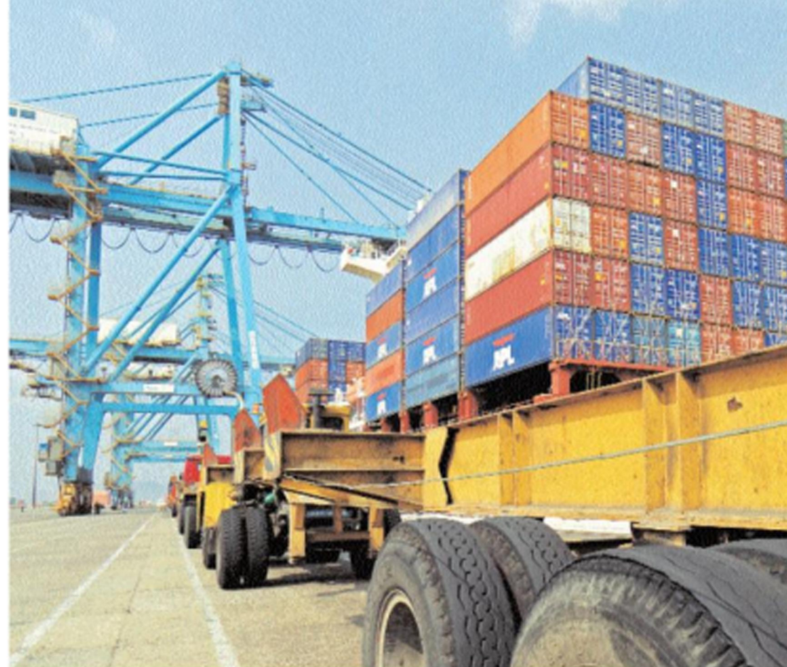
1 TRACTOR-TRAILERS LINE UP TO OFFLOAD CONTAINERS AT THE RAIL-MOUNTED QUAY CRANES ON THE QUAY AT JN PORT
