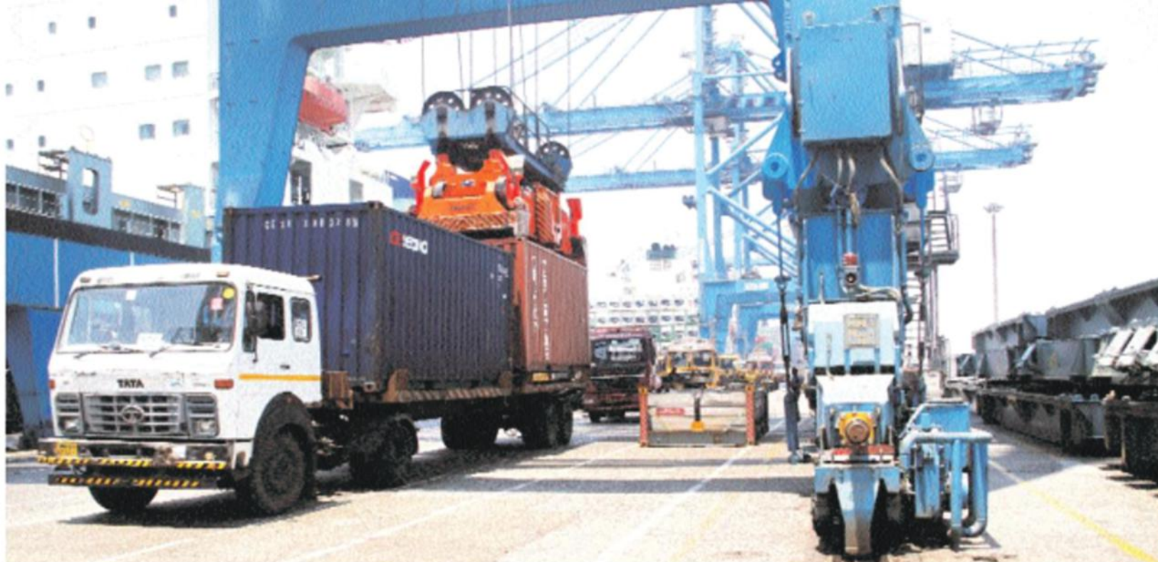
L A 'SPREADER' GRIPS AND LOWERS A CONTAINER ONTO A TRACTOR-TRAILER AT THE PORT-OWNED AND OPERATED CONTAINER TERMINAL.
