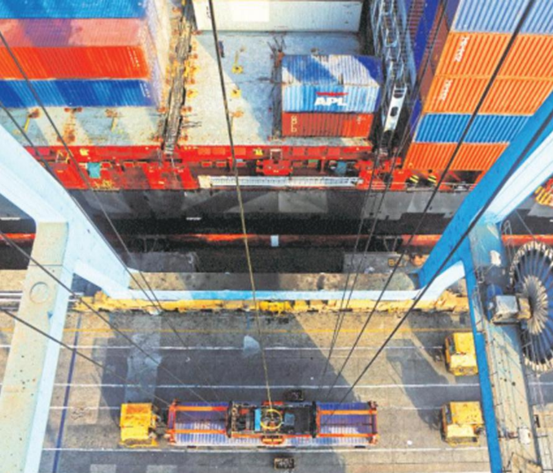
1. TOP VIEW OF CONTAINERS BEING DEPOSITED ON A TRACTOR-TRAILER FROM THE VESSEL HOLD. THE SPREADER (PICTURED) THAT HANGS AT THE END OF A CRANE'S STEEL WIRES CLAMPS DOWN ON THE CONTAINER WHILE IT IS LIFTED AND LOWERED.
