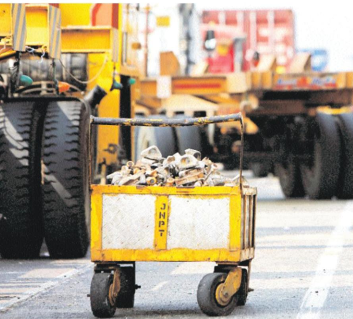
▲ A CART FOR 'TWIST-LOCKS', THAT ARE USED TO KEEP CONTAINERS IN PLACE ON A VESSEL OR ON A TRUCK
