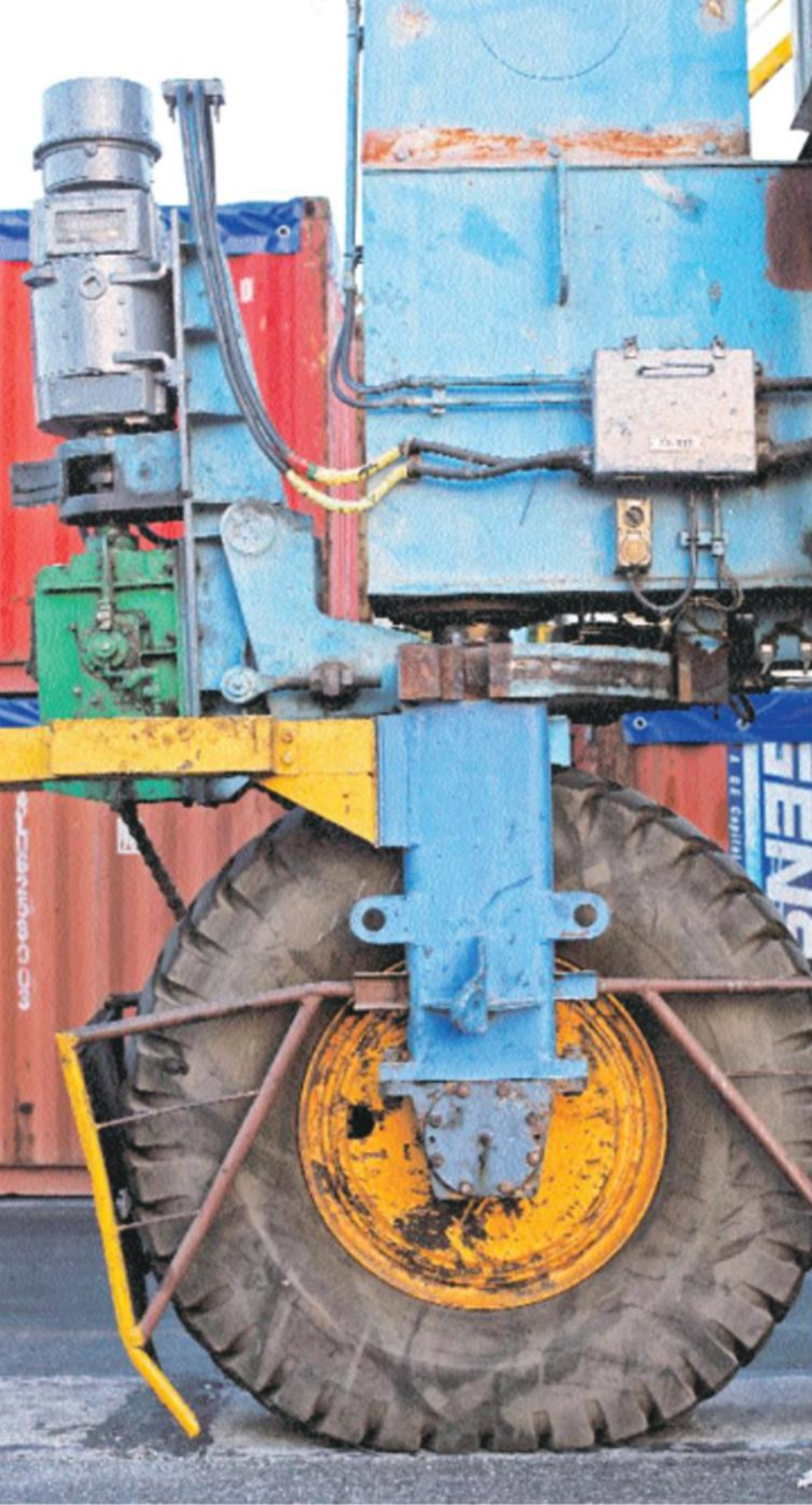
← DETAIL OF A RUBBER-TYRED GANTRY CRANES, USED FOR TRANSPORT OF CONTAINERS TO AND FROM A YARD
