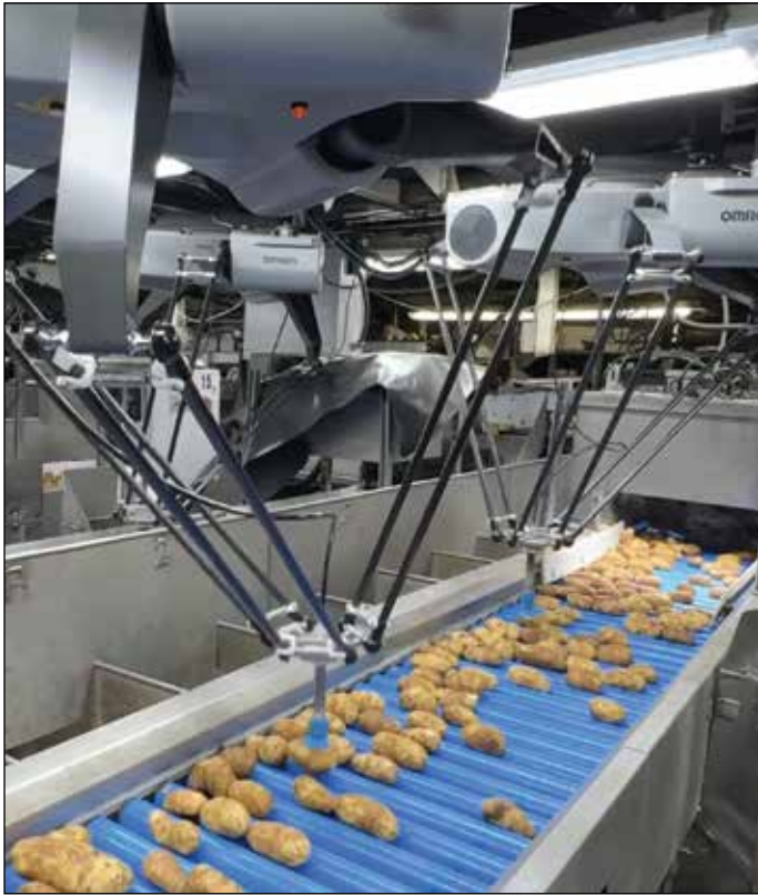
The SiftAI technology triggers robotic sorting arms to remove unacceptable products at rates up to 80-100 picks per minute with two-robot systems, as shown here.
