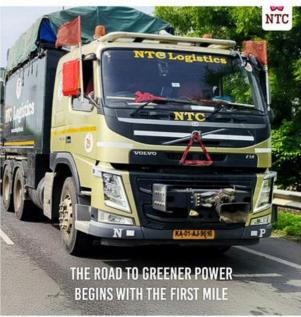
NTC Logistics is transporting a 315 MVA transformer filled with ester oil – weighing 163 metric tonnes and measuring  $8.65 \times 3.94 \times 4.66$  meters – from Maneja, Gujarat to Bhiwadi, Rajasthan, using an 18-axle configuration.
