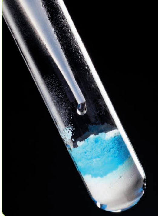
Δ Fig. 6.16 When hydrated copper(II) sulfate crystals are heated they turn from blue to white. The reaction can then be reversed by adding water.
