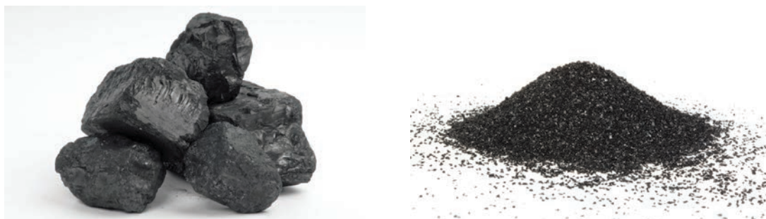
Δ Fig. 6.13 Powdered carbon has a much larger surface area than the same mass in larger lumps.
