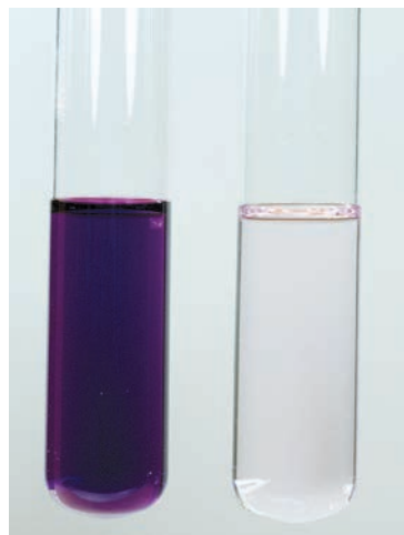
Δ Fig. 6.24 When manganate(VII) ions are reduced, colourless \text{Mn}^{2+} ions are formed.
