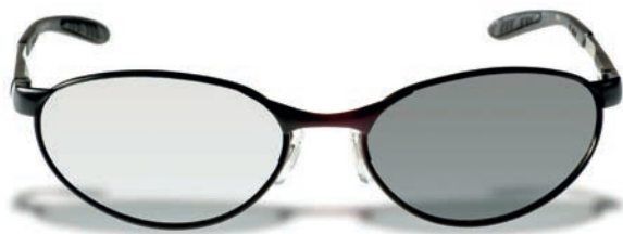
Δ Fig. 6.25 A photochromic reaction was produced when the right lens of these glasses was exposed to bright light.
