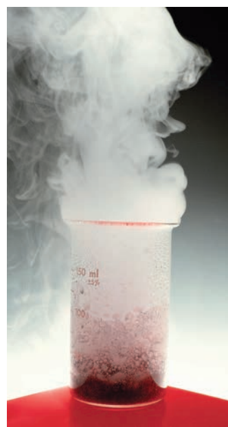
Δ Fig. 6.15 The effect of manganese(IV) oxide catalyst on the decomposition of hydrogen peroxide.
