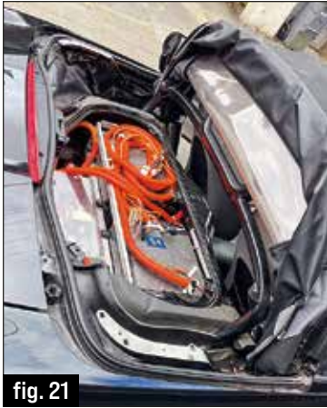
Figure 21 - Battery Box & HV cables on car
