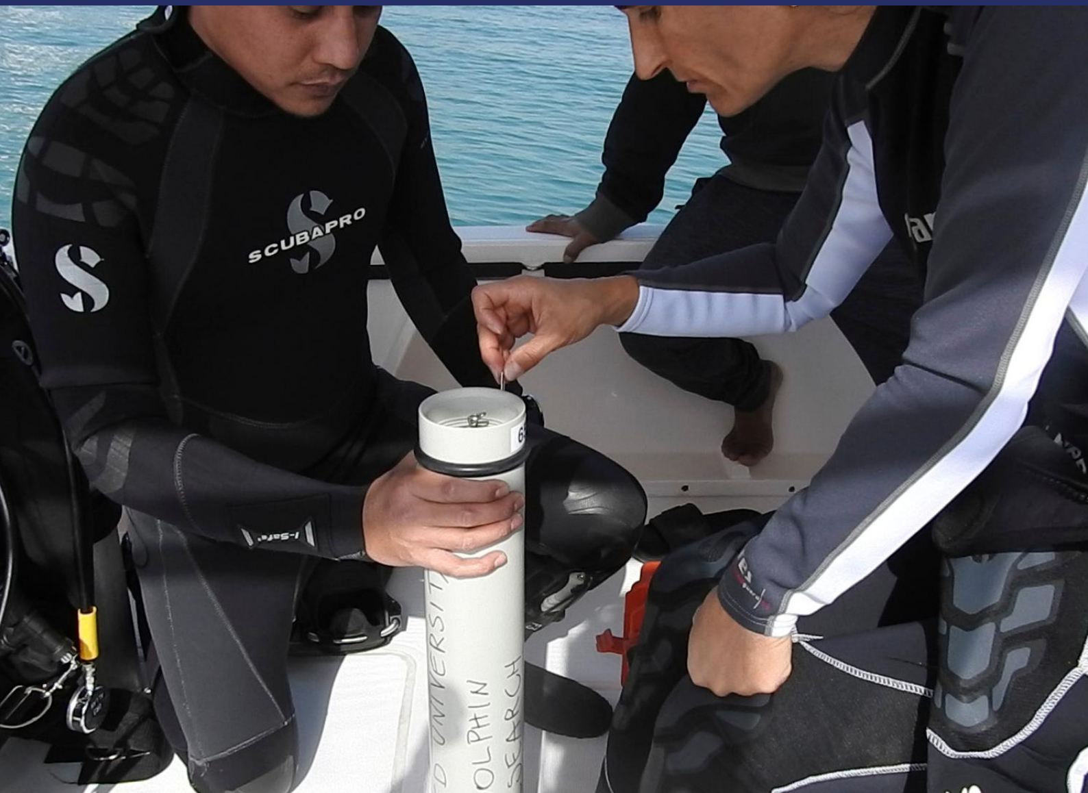
ABOVE & OPPOSITE: Fig 1. F-Pods deployed in Dubai waters. These simple, self contained but sturdy devices, can be deployed up to 100m depths. The plastic tube contains the batteries and all the technical parts to support the recording on a small SD card that when inserted, initiates the recording. OPPOSITE BOTTOM PAGE: Fig 3. Indian Ocean humpback dolphins close to Jebel Ali are recognisable for their characteristic hump supporting the small dorsal fin. They generally travel in small groups and favour waters very close to the coastline. Their population structure, and home range is still unknown.
