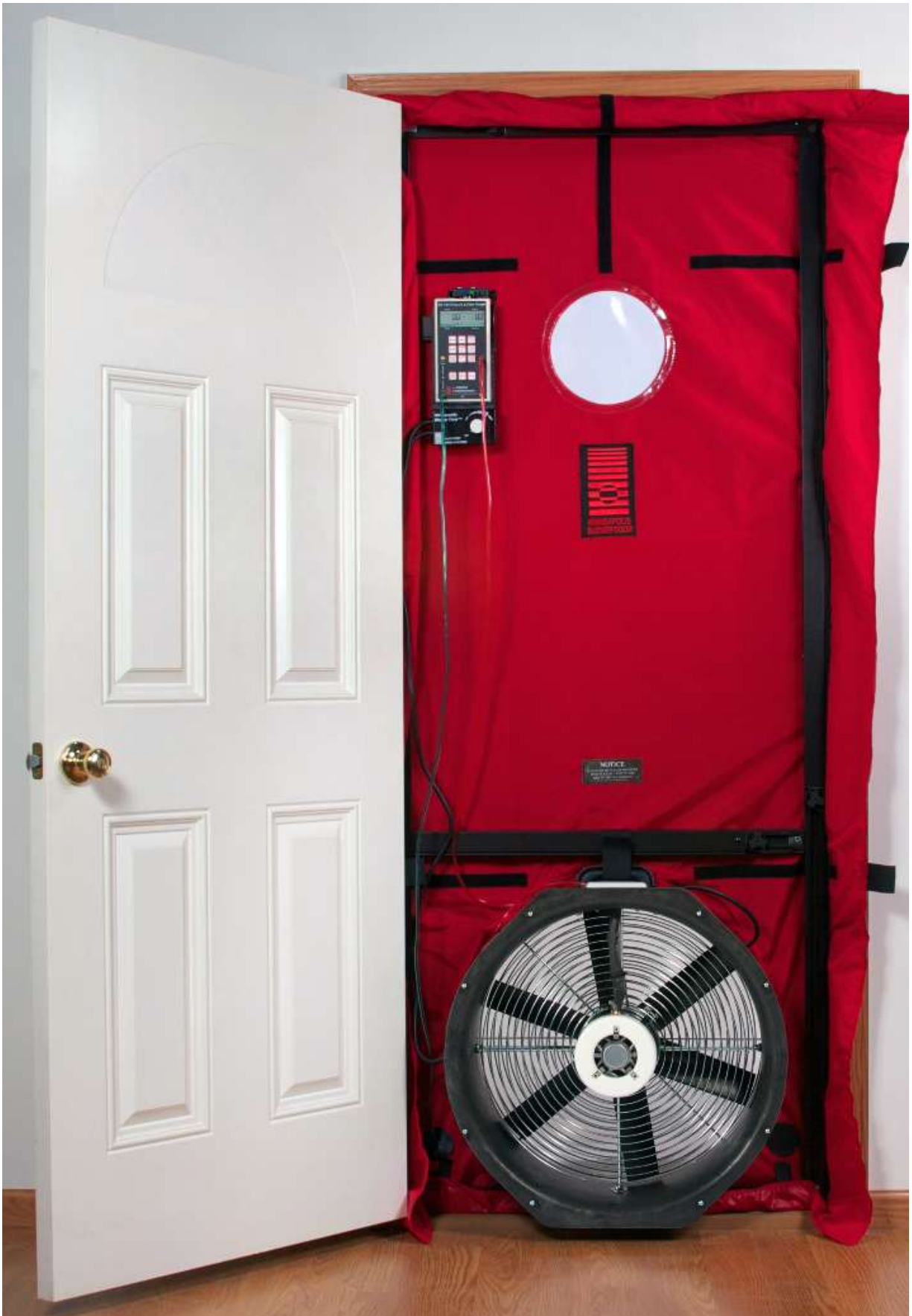
Figure 14: Blow Door Test (Wikiimedia.org).
