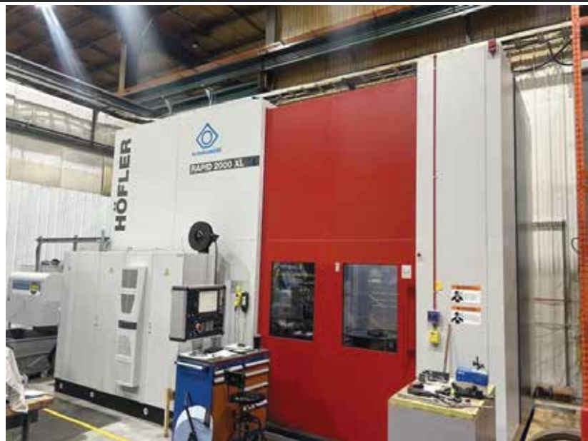
The Höfler 2000 XL is perfectly suited for the oversized gears commonly required in potash mining machinery.
