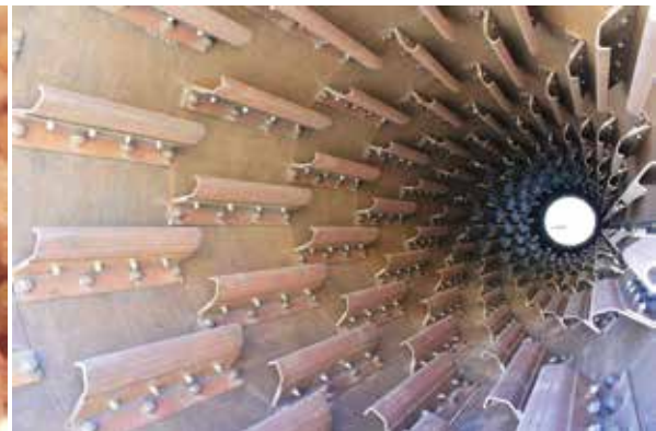
Flights in a rotary dryer.
