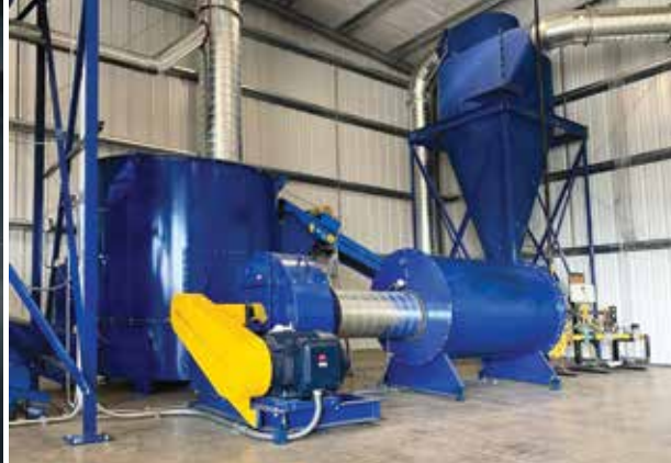
Potash dryer testing in progress in the FEECO Innovation Centre.
