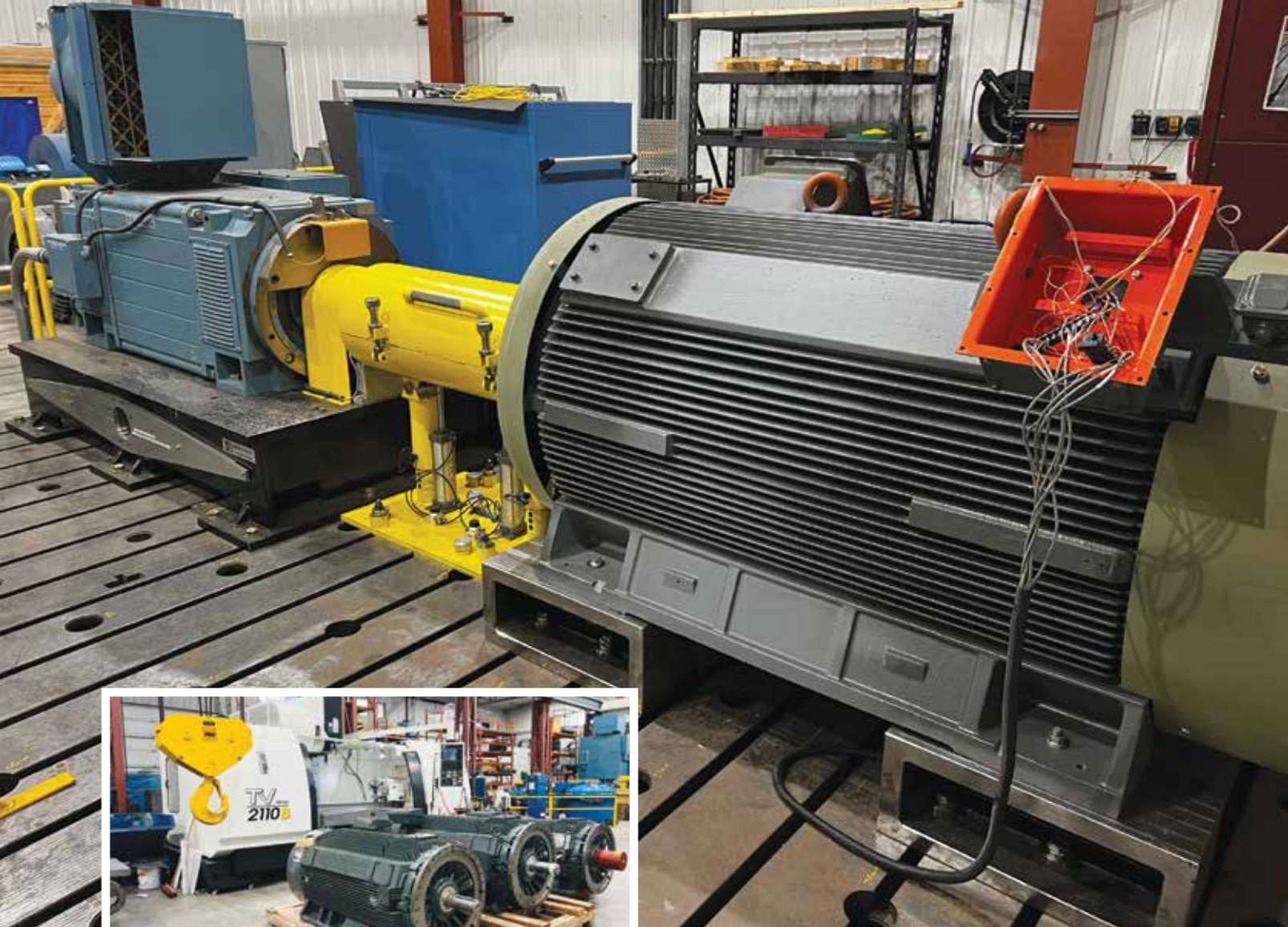
Above: Full load dynamometer test of 1200 HP repair. Inset: WEG Miner Head Motors for Prairie Machine Xcel72A Boring Miner.
