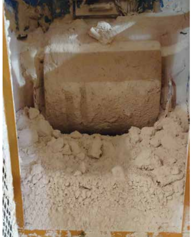
KCL build up in roll compactor.
