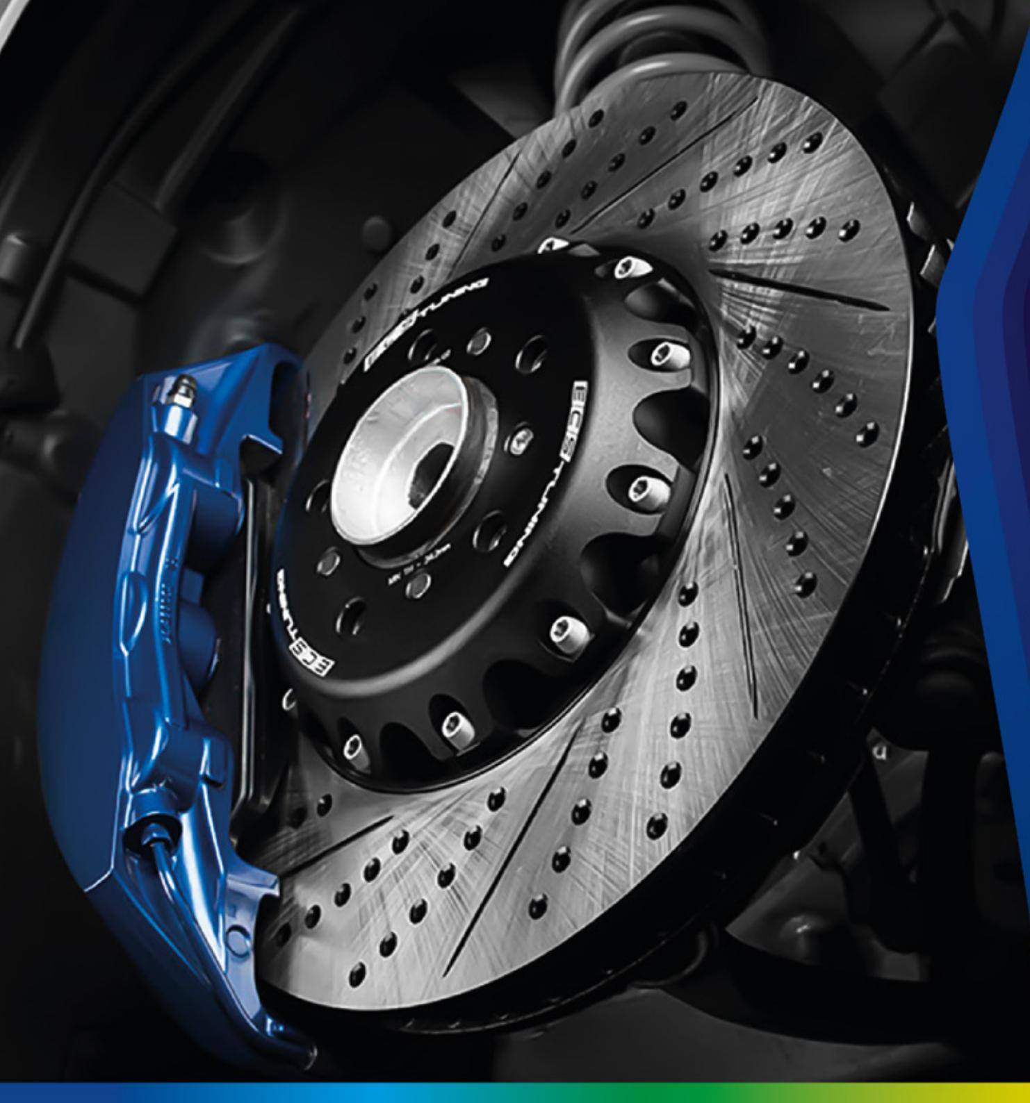
A close-up photograph of a high-performance car's front wheel assembly. The brake caliper is a vibrant blue color, which stands out against the dark, polished metal of the multi-hole perforated brake disc. The disc shows signs of use with some light scratches and discoloration. The central hubcap features the letters 'S' and 'E' in a stylized font, with '503' visible at the bottom. The background is dark and blurred, focusing attention on the wheel.
