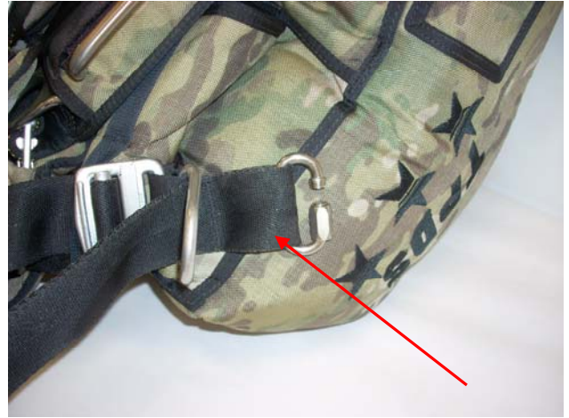
Pass the strap through the slot of the RW-8 Harness Ring of the lower Left Side of the TPDS LLT.
