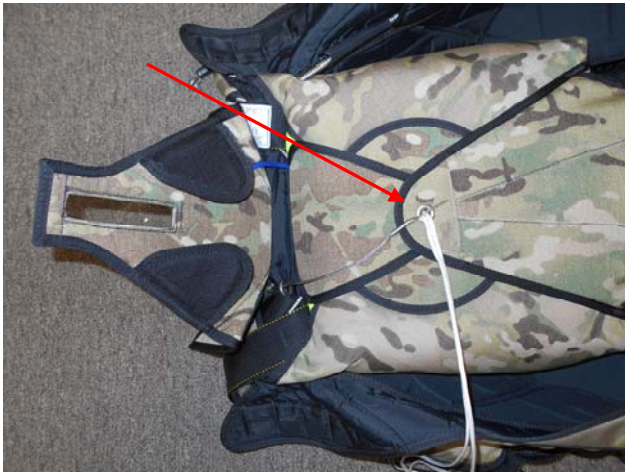
Close and secure the Bottom Closing Flap with the Reserve Ripcord Pin.
