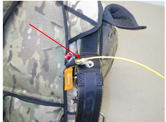
From the back side of the Riser pass the loop through the housing grommet.
