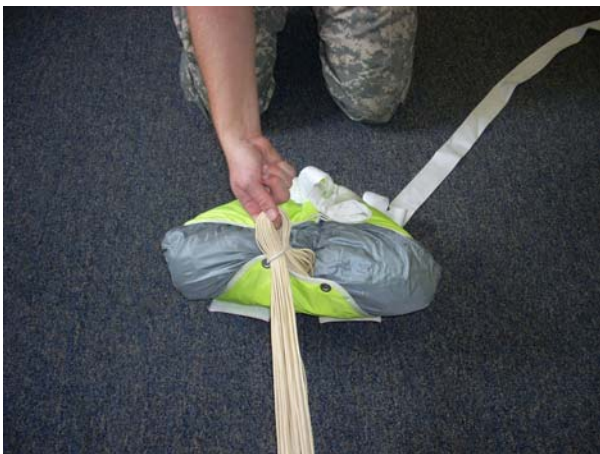
Close the Free-bag by passing the safety stow through the grommets of the Free-bag and make the first line bight approximately 1 1/2” and place in the safety stow.
