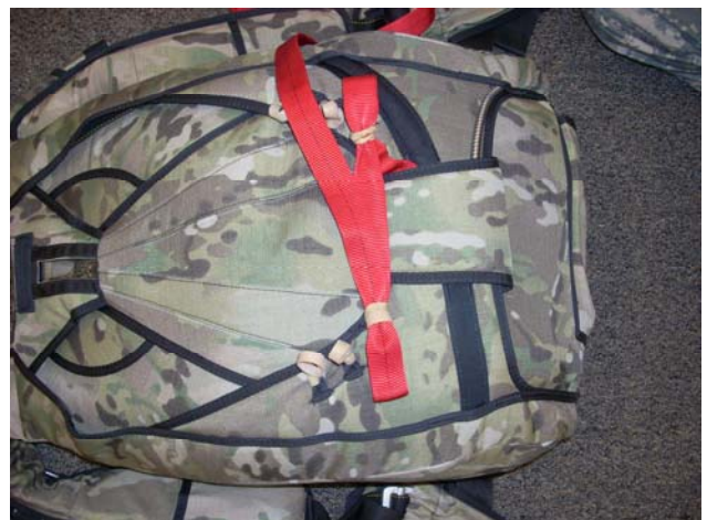
Stow the second bight of the Static Line on the Left Side of the Container.
