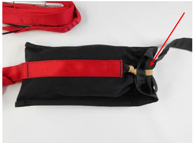
Pass the Rubber Band under the T-IV retainer and secure the Pouch closed using the rubber band and the P/C bridle as shown.
