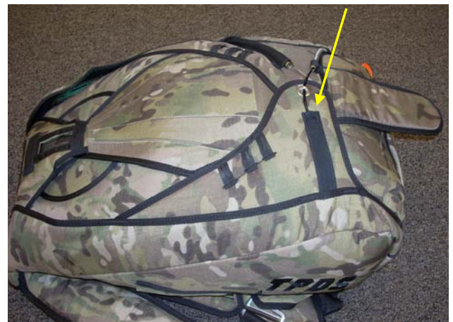
Insert the Plastic Covered Cable of the Ripcord through the closing loop then into the channel as shown.
