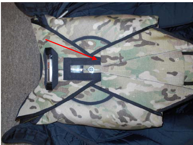
Tuck the Top Closing Flap into the slot of the Bottom Reserve Flap.
