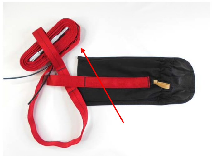
Pass the rest of the Static Line through the Static Line Loop, creating a Lark's Head Knot.
