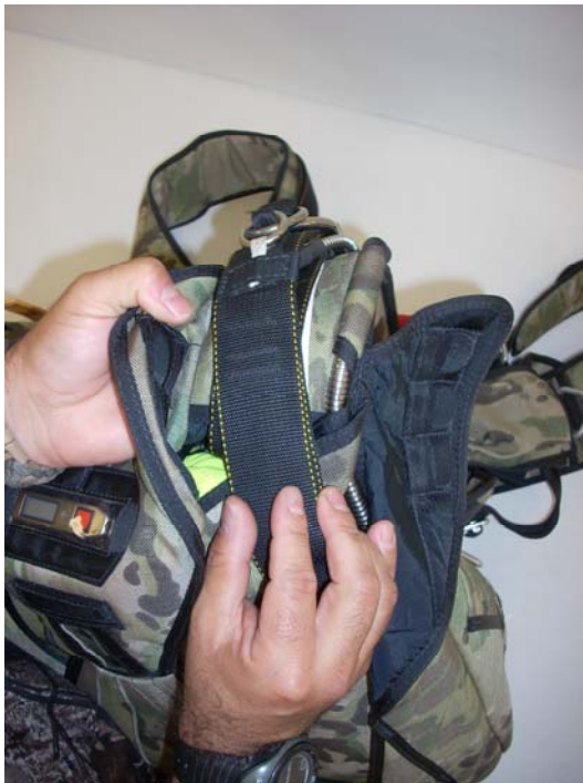
Place the Main Risers on top of the Reserve Riser Covers.
