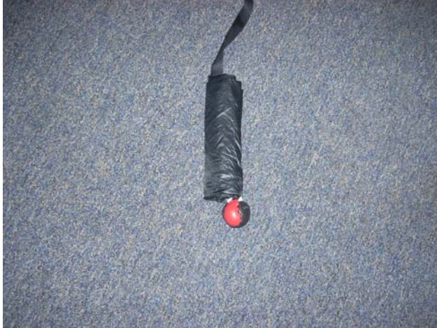
Roll the Pilot Chute into a tube.
