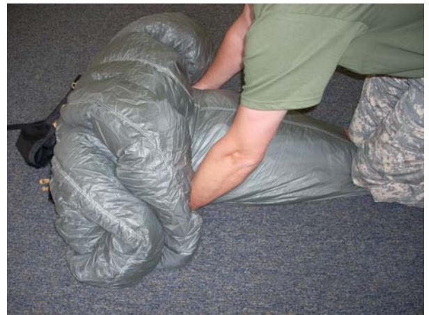
Gently squeeze the air out of the canopy.
