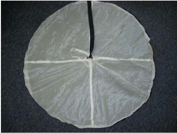
Begin laying out the Pilot Chute flat.
