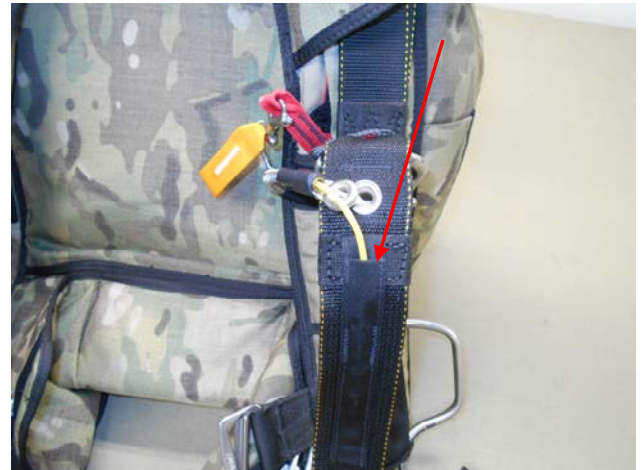
Pass the yellow cable into the T-III channel on the back side of the Main Riser.
