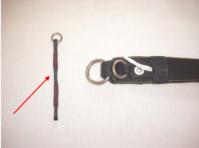
Pictured above is the Floating RSL Lanyard (TPDS-LLT-222) and the Left Side Riser.
