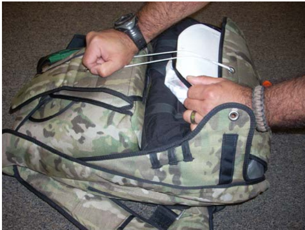
Using a short closing loop placed in the Bottom Closing Flap , close the Bottom Flap .
