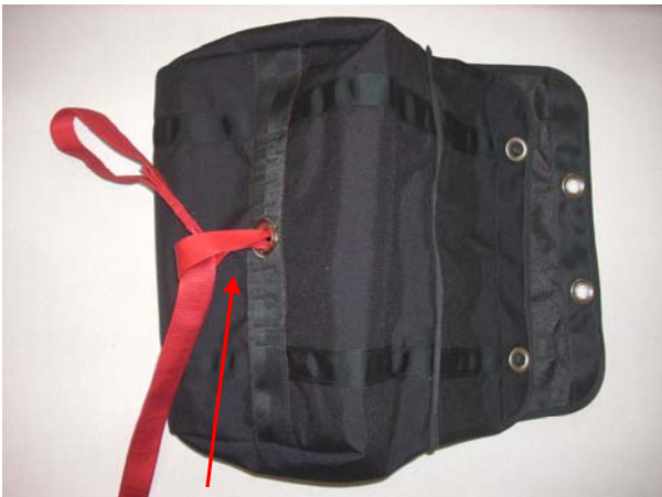
Pass the loop of the Static Line (TPDS-LLT-264) through the red loop of the Main Bag.
