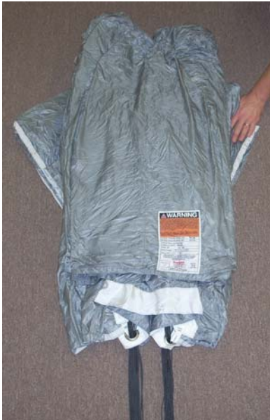
“S”-fold the four (4) nose cells under the corresponding side of the parachute.
