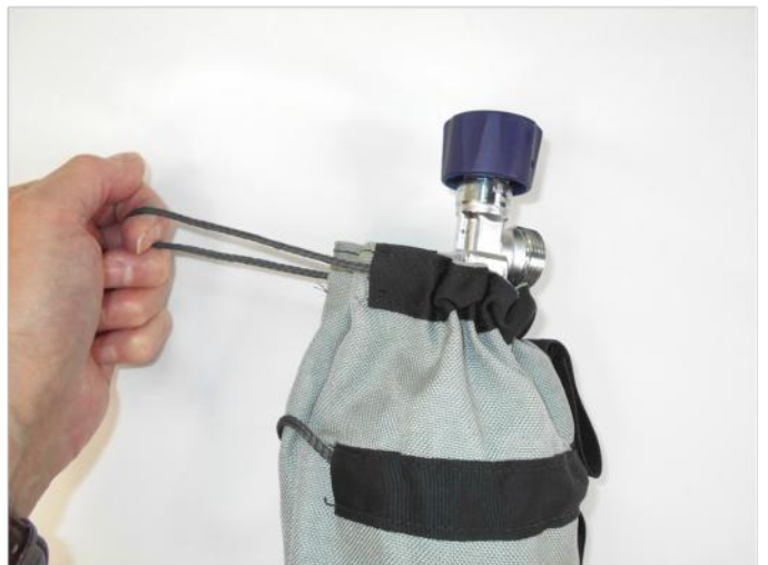
To assemble the O2 bottle holder place the oxygen bottle into the sleeve and pull the draw-string tight to close the neck of the holder.
