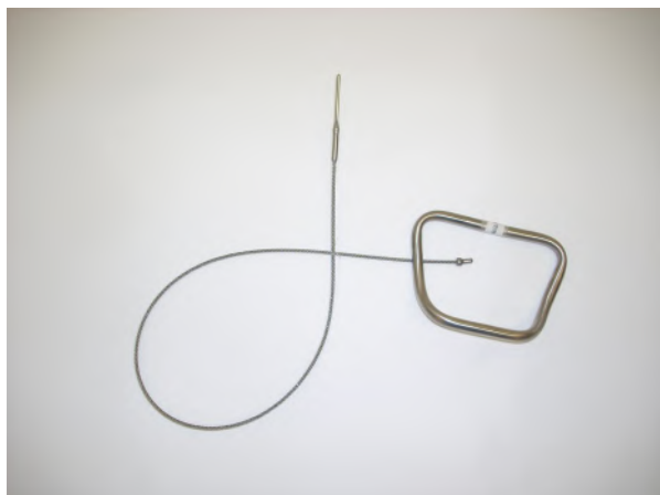
TPDS-LLT-109 Reserve Ripcord Assembly Bent Metal- Out-board
