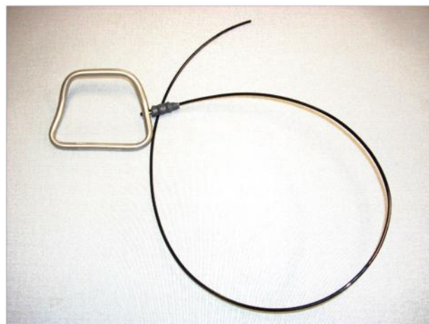
TPDS-LLT-255 Main Ripcord Handle Bent Metal- Out-board
