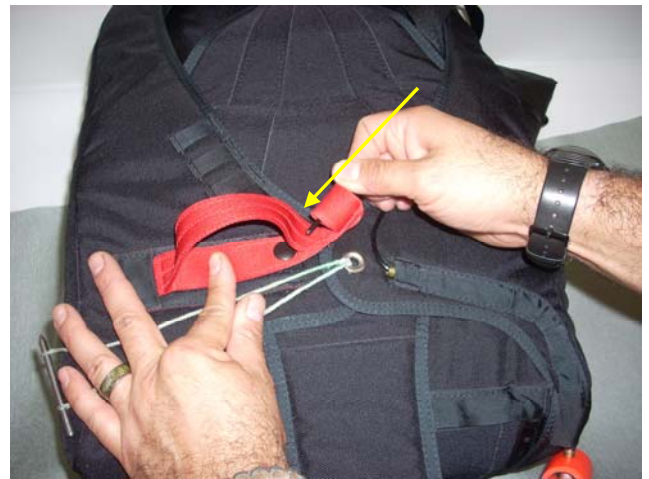
Pass the Ripcord Cable through the Loop of the AFF Jumpmaster's Handle (TPDS-LLT-266).
