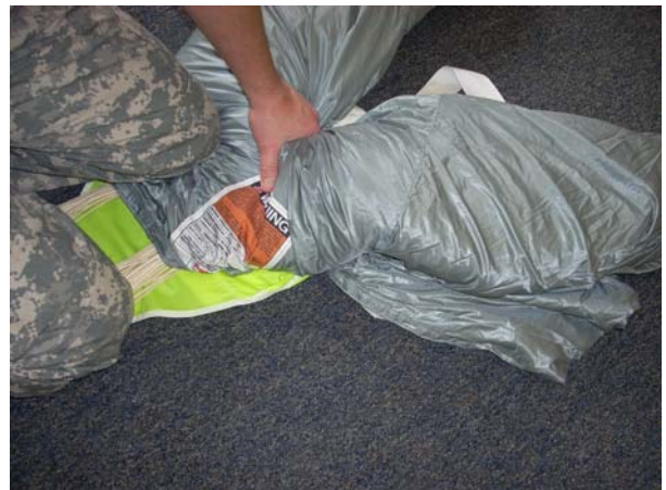
Place free-bag under the reserve with the trailing edge of the Reserve Parachute in line with the mouth of the Free-bag.
