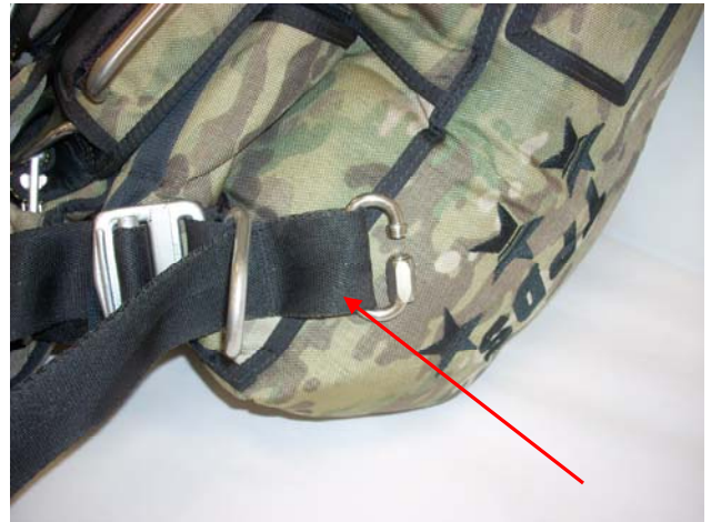
Pass the strap through the slot of the RW-8 Harness Ring of the lower Left Side of the TPDS LLT. Pass the Stainless Steel Rapide Link through the loop of the T-8 Strap.
