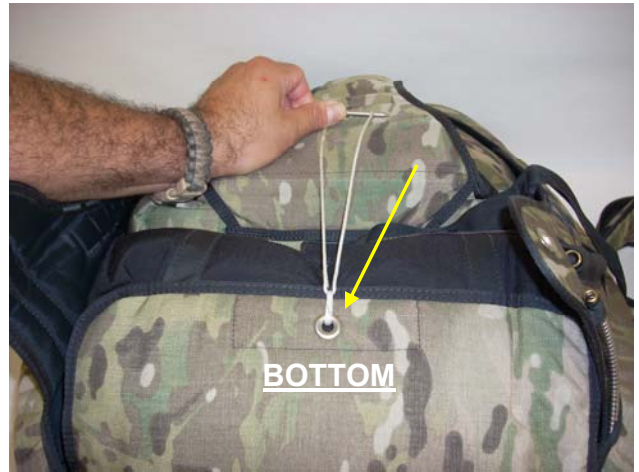
Using a closing loop on the bottom of the Reserve Container, pass the closing loop through the Bottom Main Flap .
