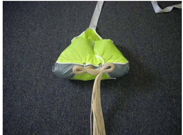
Secure the Free-bag closed by making a second line bight and placing it in the safety stow.
