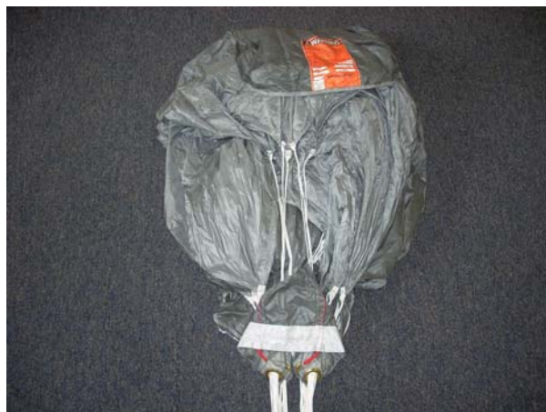
Bring the slider up from the connector links until it is touching the slider stops and quarter the slider between the slider stops.
