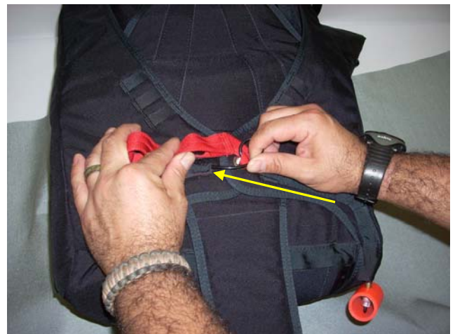
Continue to pass the Ripcord Cable into the channel on the Left Side Flap.
