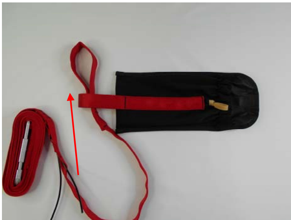
Pass the Loop of the Static Line (TPDS-LLT-265) through the Type 4 Loop on the end of the Pilot Chute Pouch.
