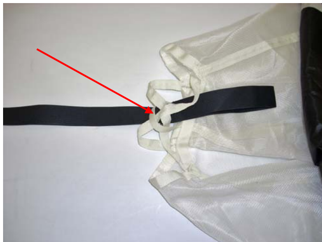
Pass the smaller loop of the Bridle (TPDS-LLT-245) through all of the Pilot Chute (TPDS-LLT-231) Loops.
