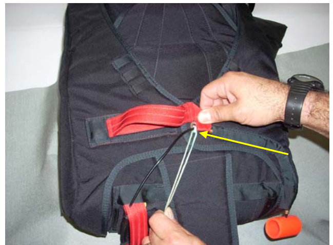
Pass the Ripcord Cable through the Closing Loop.
