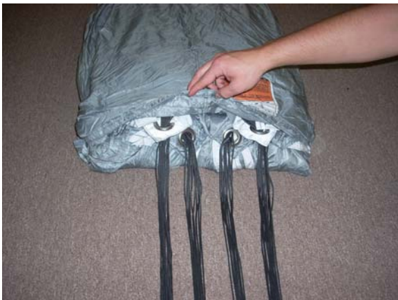
“S”-fold lower portion of canopy up to the trailing edge of the parachute and place under the trailing edge. If Needed.
