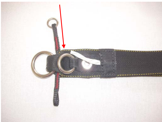
From the inside of the Left Riser pass the end loop of the TPDS-LLT-222 through the riser between the two webbings.
