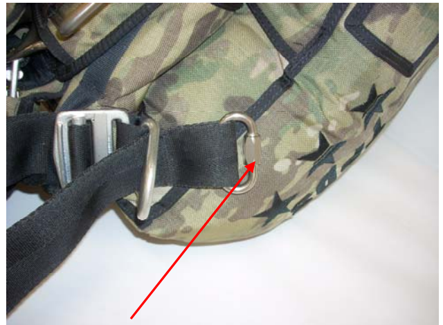
Tighten the nut "finger tight".
