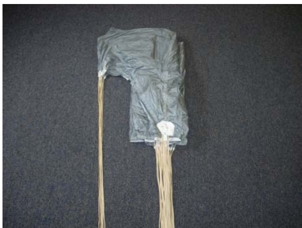
Grasp the D-line group under slight tension and fold over the C-line group.
