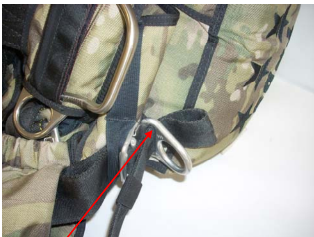
Pictured above is the other half of the Belly-Band. When installing it to the Left Side of the TPDS LLT be sure that the "turned back" end is facing the Harness/ Container to prevent it from slipping when fed through the Friction Adapter.
