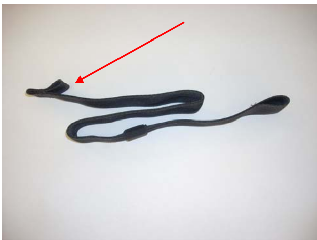
Pictured above is the other half of the Belly-Band. When installing it to the Left Side of the TPDS LLT be sure that the "turned back" end is facing the Harness/ Container to prevent it from slipping when fed through the Friction Adapter.
