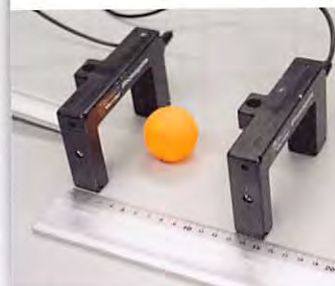
A.1 Figure 6 The ball interrupts the infrared light transmitted across each gate as it passes through them. The times of these interruptions are measured and recorded by a data logger.
