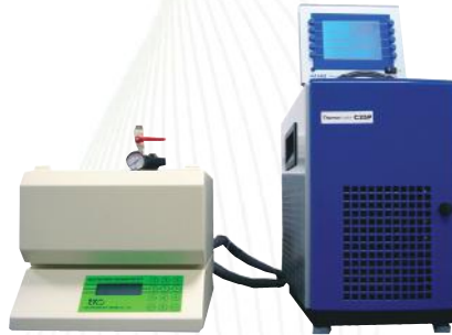
K-Factor Machine Measuring the thermal insulation properties of polyurethane foam systems.
