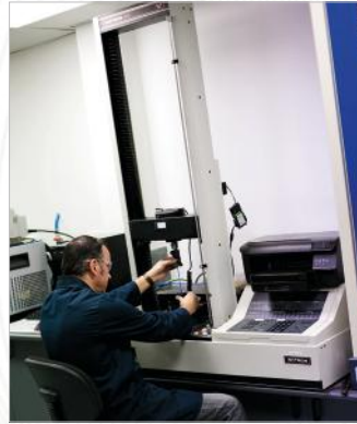
Tensometer Testing a range of tensile related properties, including tensile strength, elongation and tear strength.
