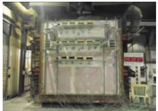
One of our numerous fire tests, all variants penetrations being tested uncapped/uncapped (u/u).
