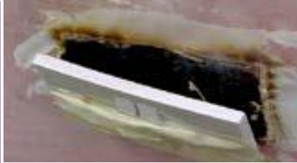
FireSure® Gasket after fire test. Note the gasket has completely filled the box and the layers of plasterboard including covering the gaps around the edge of the box.
