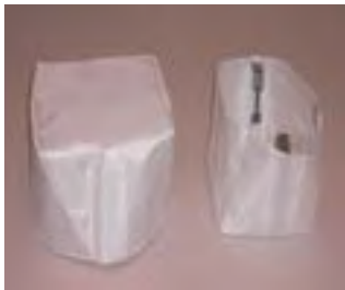
FireSure® Intumescent fire and acoustic covers before and after fire test. Fixed in place using attached clamping brackets. No tools required.
