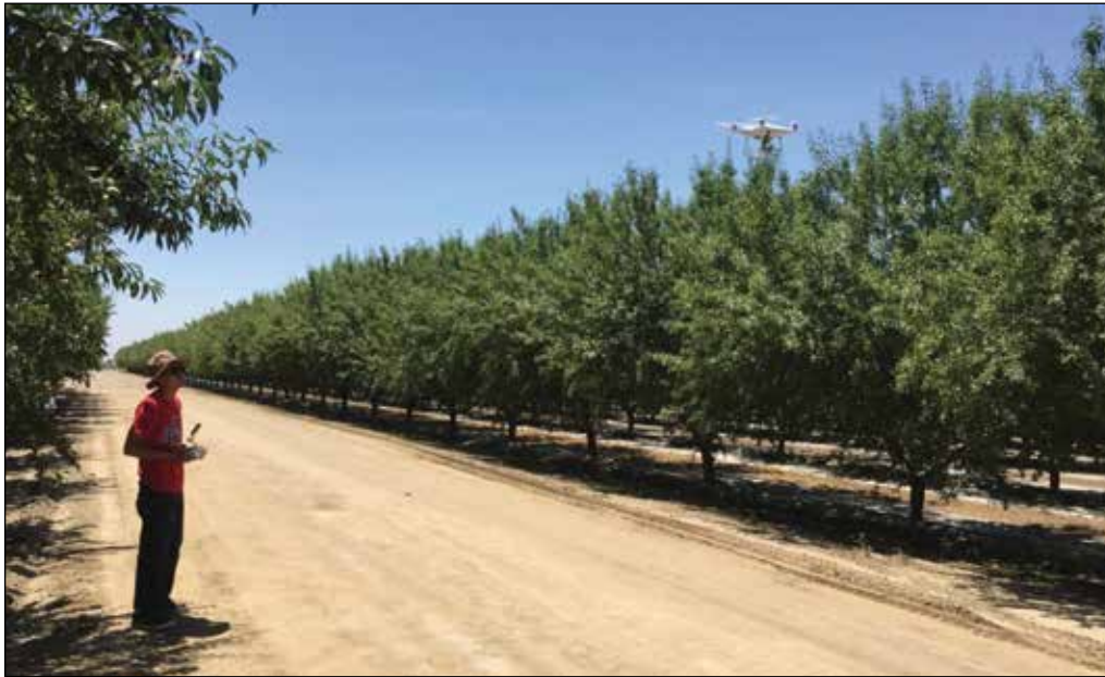
Unmanned aerial vehicles, or drones, can help farmers monitor the state of fields and orchards but data can be affected by the position of the sun. A web application developed at the UC Davis Digital Agriculture Lab helps farmers and researchers find the best time to fly for their date and location to avoid creating errors in data. Photo courtesy of Digital Agriculture Lab
