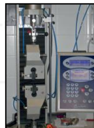
Dynamometer Tensile Stress-Strain (ISO 037) Tear Strength (ISO 034-1)
