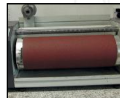
Cylindrical Drum Abrasion Resistance (ISO 4649)
