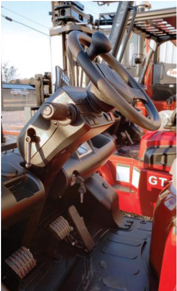
Adjustable Steering Column Pivots 30 Degrees
