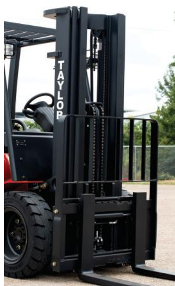
Durable Nested I-beam Design Yields Optimal Visibility
