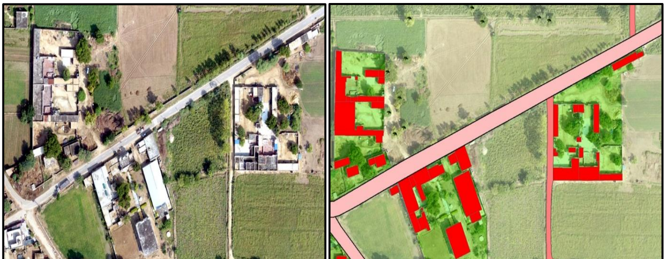
Fig 7: Ortho Rectified Image and feature extraction
