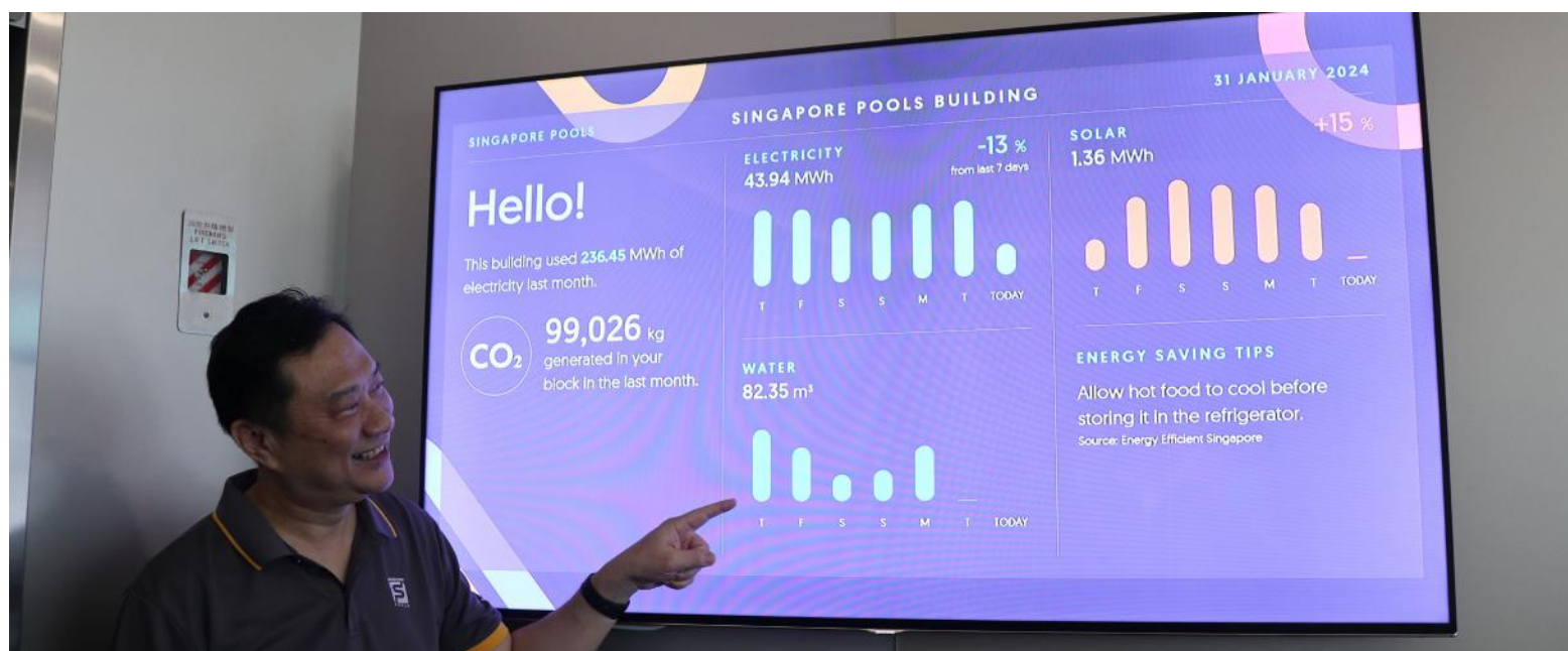
The Smart Green Dashboard is displayed at the building’s lobby and operations centre, empowering Singapore Pools employees to monitor their energy consumption and stay conscious of the environmental impact.
