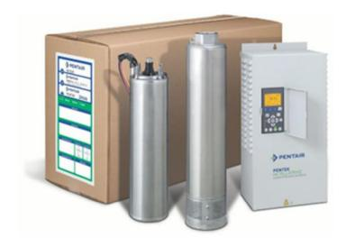
The Pentair Pentek Intellidrive Constant Pressure Controller automatically adjusts motor speeds to meet changes in water demand. Instantaneous feedback from an electronic pressure transducer instructs the drive to change the submersible well pump motor speed to maintain constant pressure throughout the system. Available in various sizes.
