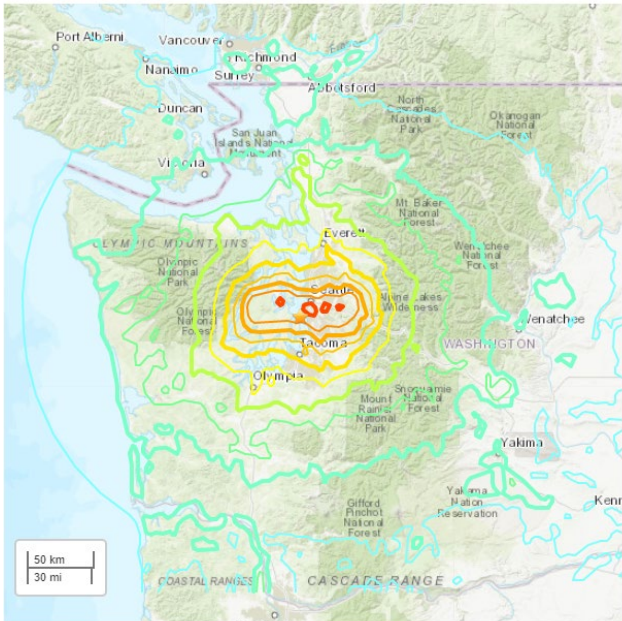
Figure 4.2-5 Magnitude 7.2 Scenario Earthquake – Seattle Fault Zone – Northern 9.0 km depth
