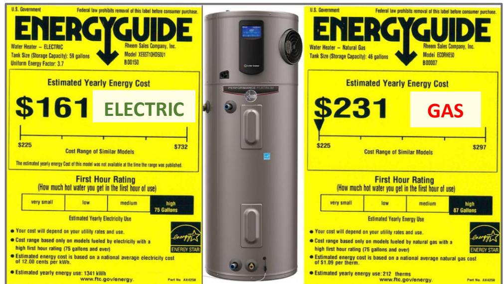
Figure 9: US Dept of Energy labels show with average U.S. energy prices, heat pump water heaters cost $70 per year less to operate than the most efficient gas water heaters on the market.
