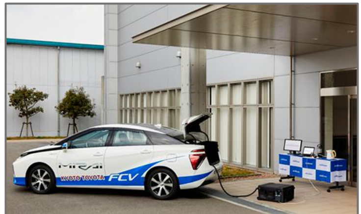
Figure 27: The “Power Mover” a 4.5kW portable EV power station that can also supply typical AC appliances. 77
