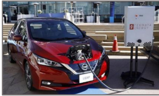
Figure 23: Nissan unveils the U.S. commercial offering of V2H charging in LA for 2019 deployment in the U.S., using battery-powered Leaf cars and Fermata Energy bi-directional charging. 71
