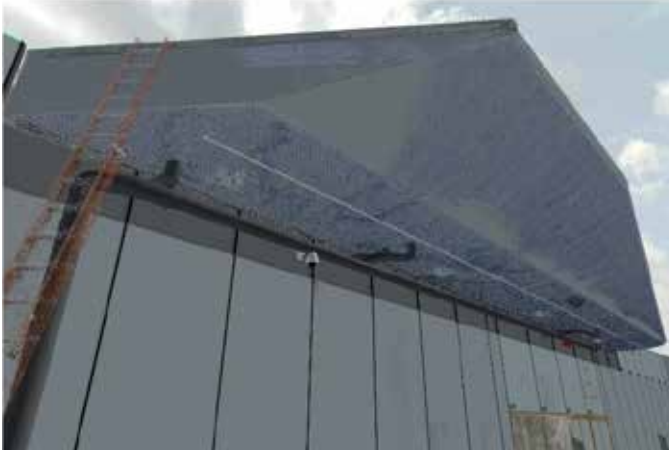
Image 6 – Canopy point cloud overlaid to the 3D model.
