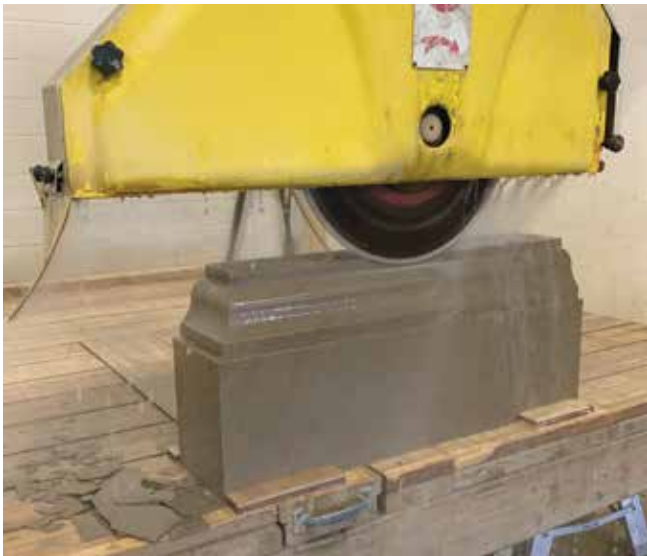
CNC machine stone profiling with saw blade and router bit.
