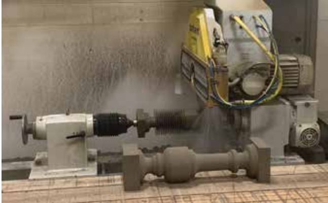
Turning main roof baluster on lathe.
