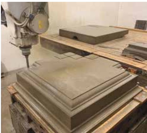
CNC machine stone profiling with saw blade and router bit.
