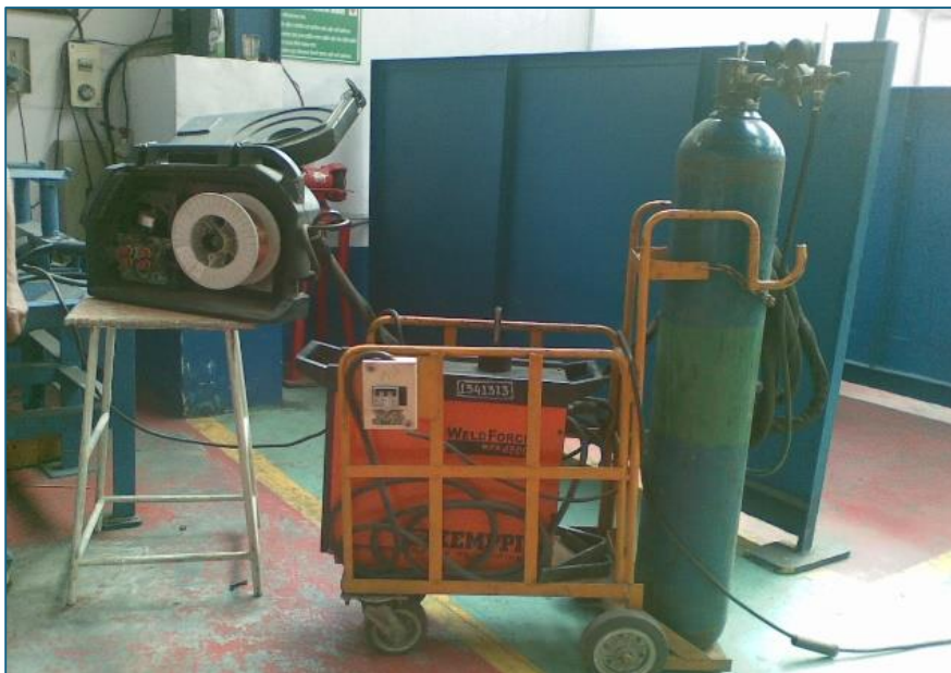
Figure 4: Wire Feeder, Inverter, Cylinder for Gas Storage
