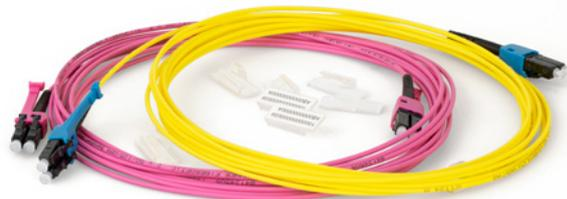
Duplex assemblies, also called duplex patch cords, are 2-fiber cables terminated with LC duplex connectors on both sides. In the last five years LC has become the most popular connector in the world, especially in the white space.
