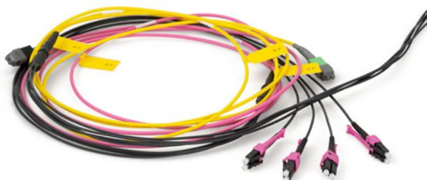
Harness cables are in-rack single jacketed cables with a MTP Pro connector at one end and four duplex connectors on the other end. They are supposed to directly connect one parallel transceiver to four duplex transceivers (so called breakout mode) located in the same rack.
