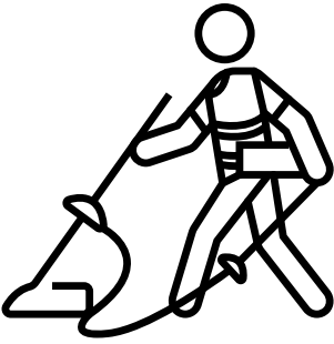
High-frequency impulse radar (up to 0.5m depth) to scan reinforcement.
