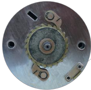
Safety brake with two pawls
