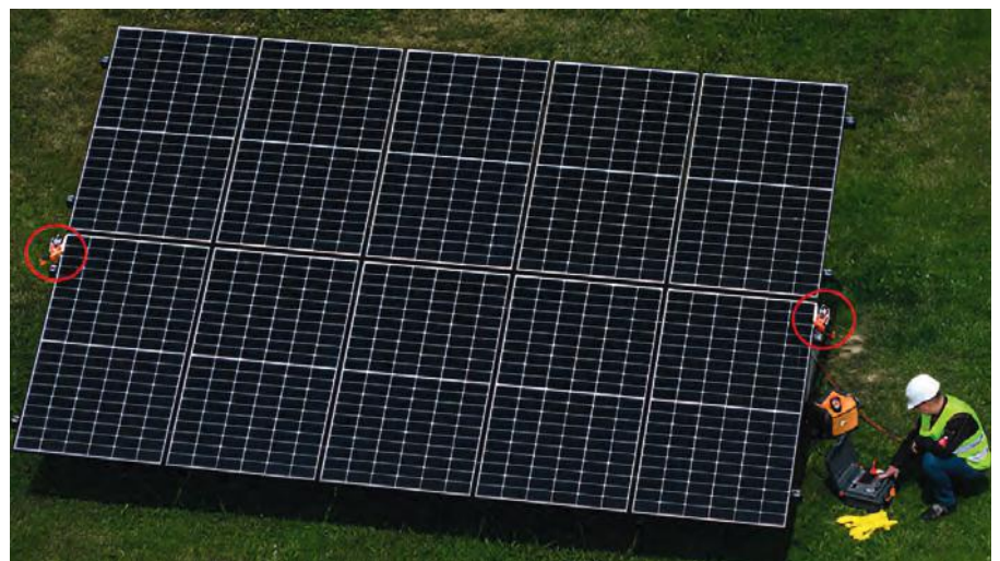
Two irradiance sensors at both ends of the PV string
