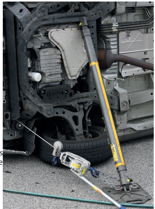
Contrast the main picture’s modern, All-in-One strut, in the form of Holmatro’s V-struts, with the traditional tensioned buttress solution using ladders. This will always work in a pinch but much better to have the speed, efficiency and firm placement of a purpose-built All-in-One strut.
