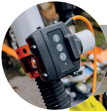
Holmatro remote controller and multi-strut load sensor. Above-left: Holmatro single strut powered extender
