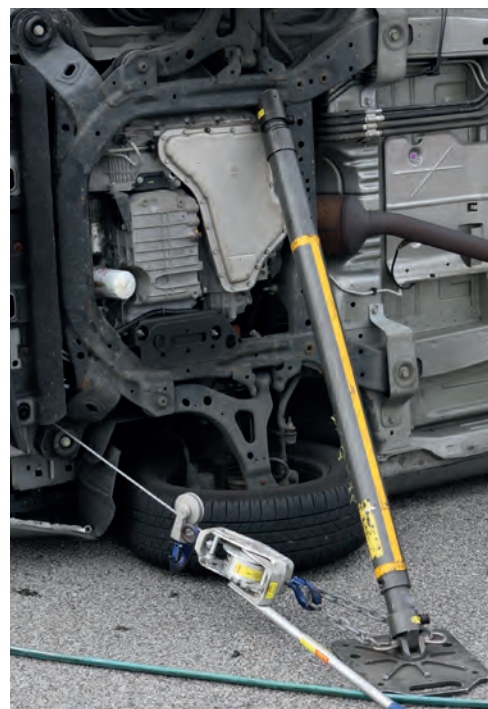
Contrast the main picture's modern, All-in-One strut, in the form of Holmatro's V-struts, with the traditional tensioned buttress solution using ladders. This will always work in a pinch but much better to have the speed, efficiency and firm placement of a purpose-built All-in-One strut.
