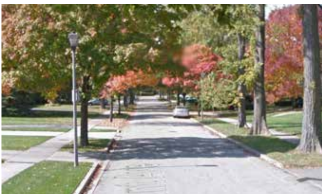
Example of 50 ft wide right-of-way. Source: Claremont Ave, Elmhurst IL - Google Streetview
