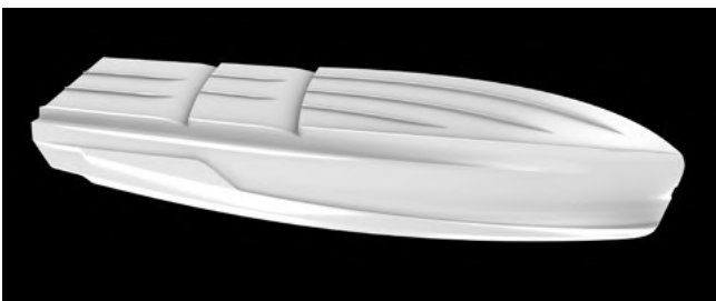
A Rhino3D rendering of the inverted hull shows the step and strake configuration.
