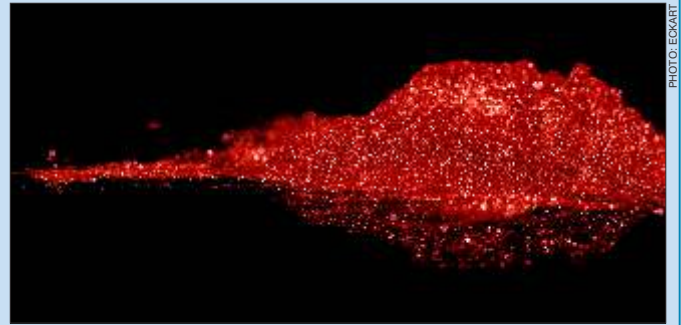
Compared to the already successfully launched LUXAN CFX C842 Spotlight Red, the new LUXAN CFX B842 Immersion Red has a more subtle effect, a smoother clear coat level and a reduced graininess.
