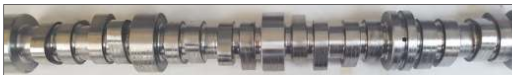
Camshaft protected by EcoLine® 3690 after four days in salt spray conditions.
