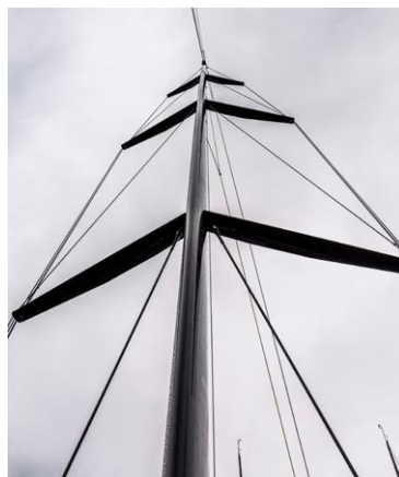
RIG: The RC44's carbon fibre mast comes in two pieces to facilitate transportation. Its standing rigging is in continuous Future Fibres PBO.
