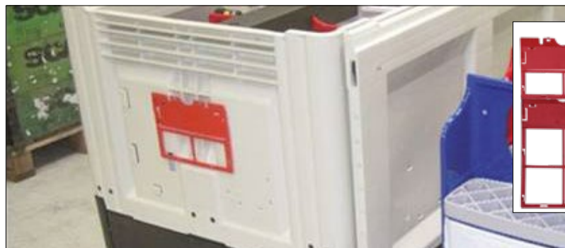
Space saving ratio at 805 mm height 3:1, at 978 mm height 7:3.
