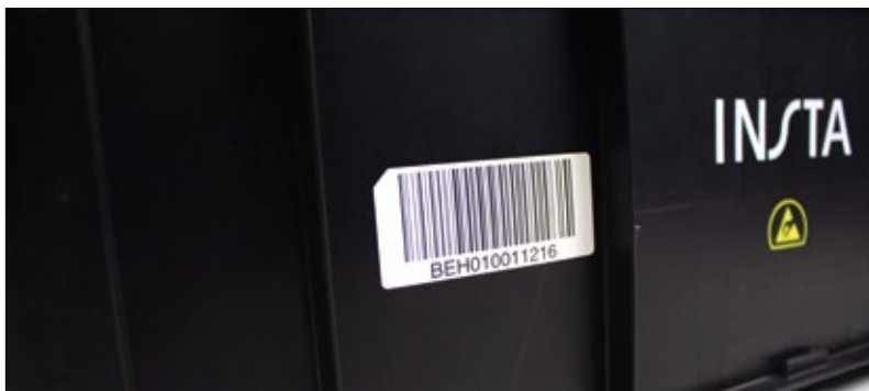
A non-removable barcode on a container by means of in-mould labelling.
