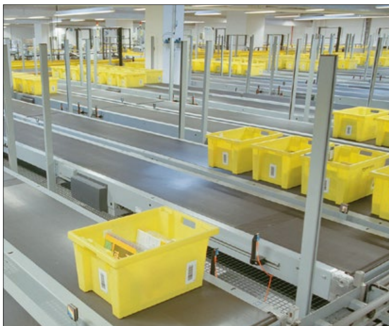
Bins with reinforced bases on a distribution system for e-fulfilment. (Photo: Vanderlande Industries)
