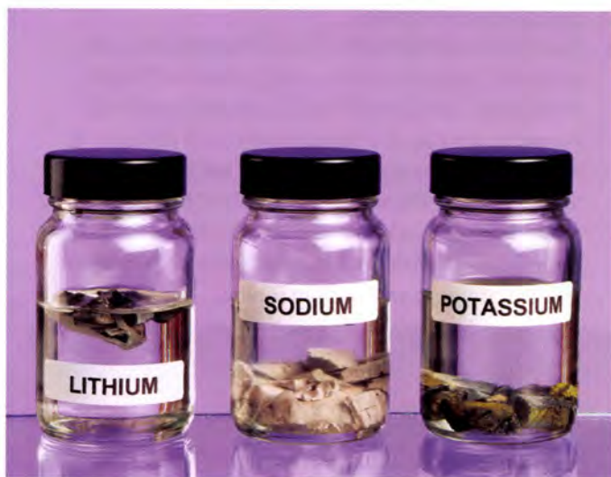
■ Figure 3.14 The alkali metals need to be stored in oil to prevent them from reacting with the oxygen in the air
