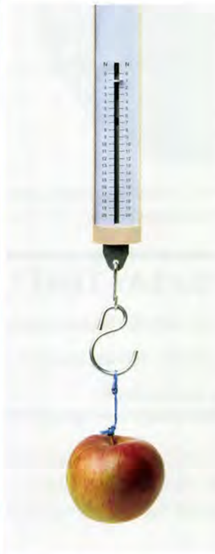
■ Figure 2.23 A force meter or 'Newton' meter (sometimes called a spring balance) uses a spring adjusted to stretch a known amount for a given gravitational force
