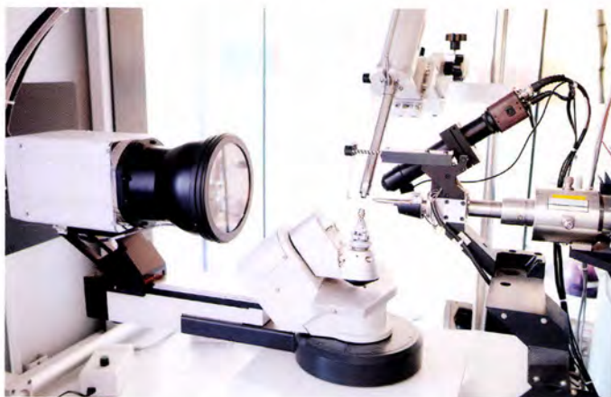
■ Figure 2.13 An X-ray crystallography machine; a crystal is held in place between a screen and a device which gives out X-rays
