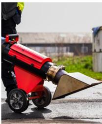
Jointline's Jet Drying Solutions provide an advanced, high-speed method for surface drying and preparation across a range of applications, including road marking, waterproofing, crack sealing, and maintenance. Our powerful jet dryers remove moisture, debris, and ice from surfaces, ensuring optimal adhesion and improved efficiency in all weather conditions.
