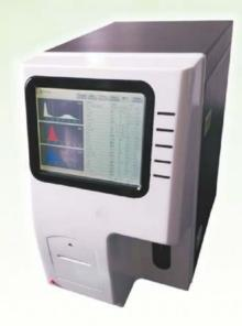
·Test principle: Impedance method for WBC, RBC and PLT.
