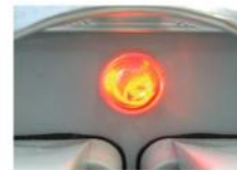
Caution (Orange blinking)
