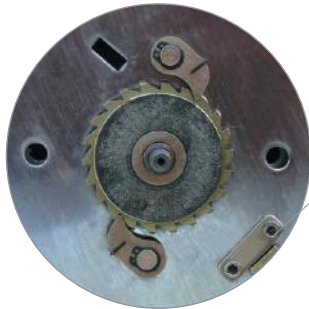
Safety brake with two pawls
