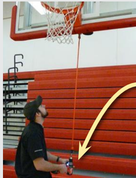
Optional BA931 Cordless Winch Winder Operation
