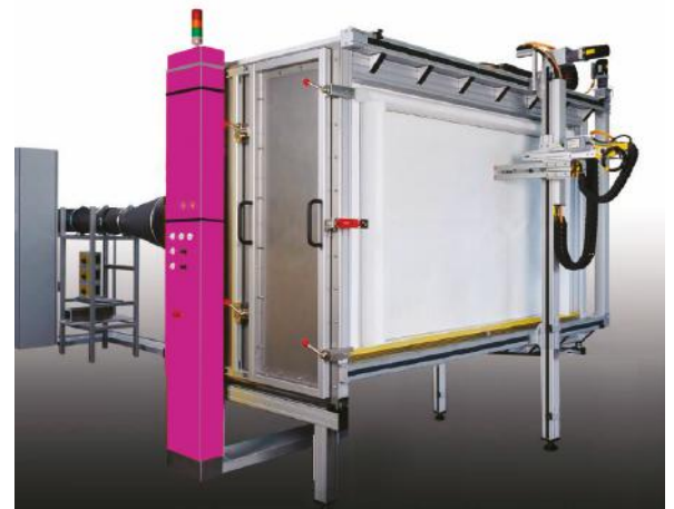
Photo : Essai de scanning - EN1822-4
