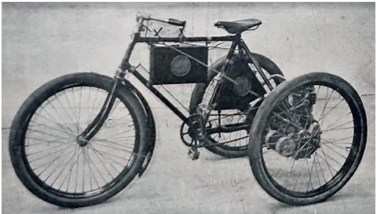
An advert for Automoto in the magazine La Vie Au Grand Air proclaimed: "This is the machine which Ducom chose for his Paris-Brest record." It was rated at 2hp @ 1,500rpm; the engine weighed 26kg.
