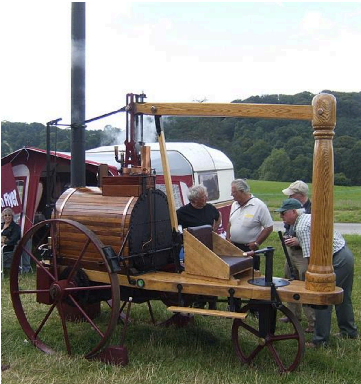
Redruth, 2004: a team of enthusiasts known as The Murdock Boys set out to finish the job and build a working steam locomotive based on William Murdock's model (or,
