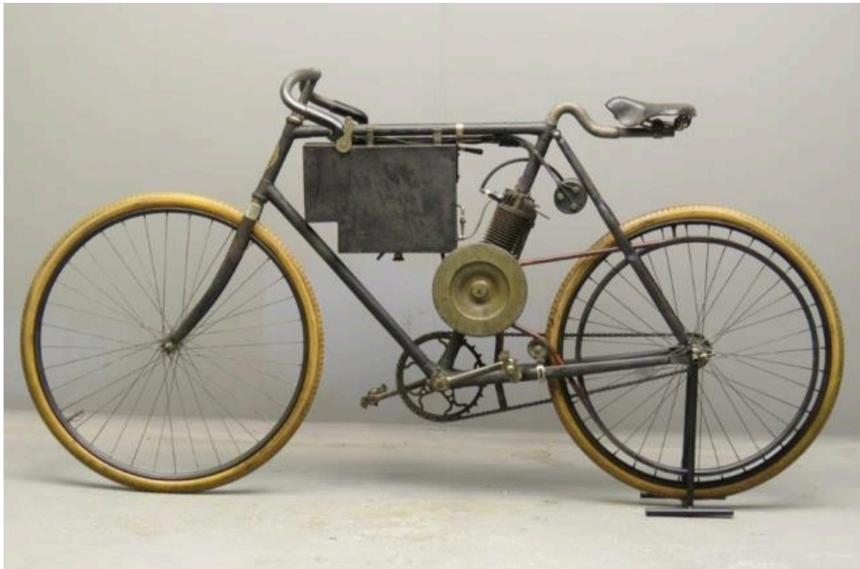
Labre & Lamaudiere of Paris developed a 64cc clip-on four-stroke engine with battery/spark ignition that span up to 2,000rpm.
