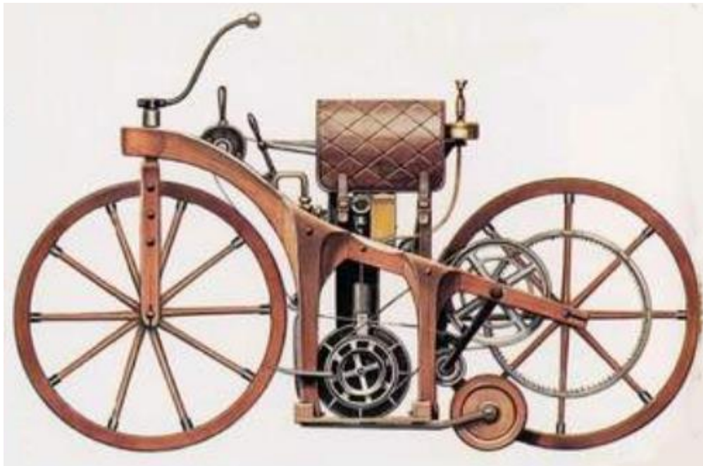
The Einspur was a short-lived testbed for a car engine, but here it is: the first motor cycle.
