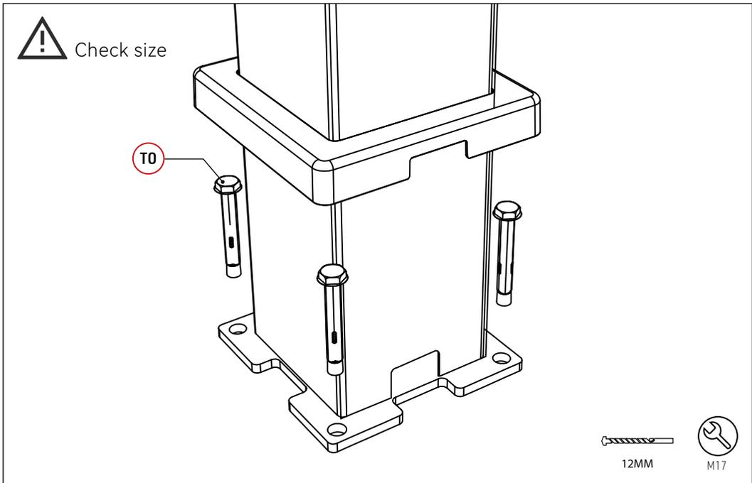
Move the bottom of the columns according to the dimensions on the front page to ensure that the dimensions are the same, then use a 12mm impact drill bit to guide the holes, then put in the expansion screws and tighten them with a M17 spanner.
