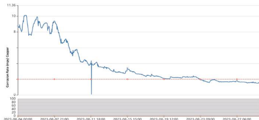
Figure 7 measurement of oxide layer deposition on copper surface.
