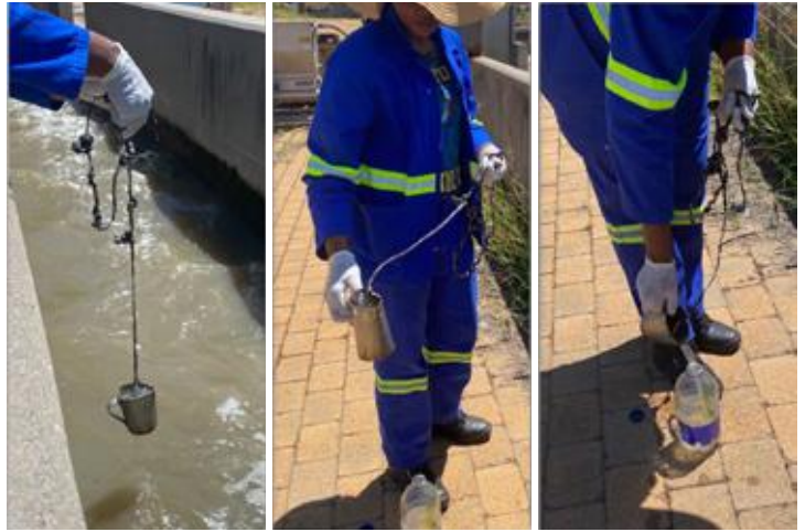
Water being collected and treated with Rubicon Eco at a wastewater treatment plant
