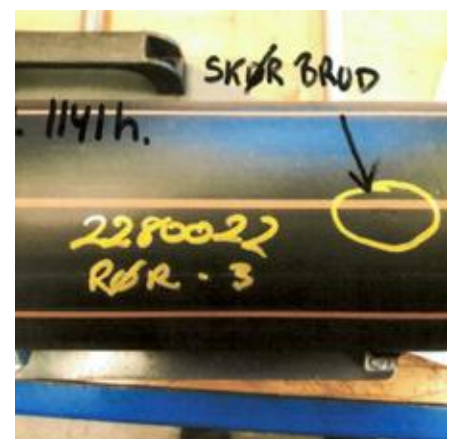
The 110 mm pipe with recycled material showed a brittle failure, this illustrates that this pipe is not suitable for pressured environments
