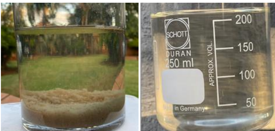
Before and after two minutes of dirty water being treated with Rubicon sachets
