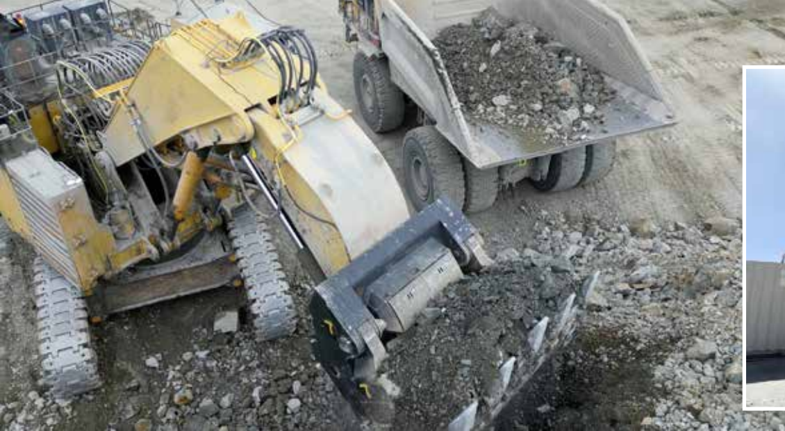
Above left: ShovelSense™ system in operation, for grade monitoring in real time as material is loaded into a haul truck. (MineSense Technologies). Inset: BeltSense™ system, which analyzes metal content on the conveyor belt for real-time grade monitoring and sorting. (MineSense Technologies).
